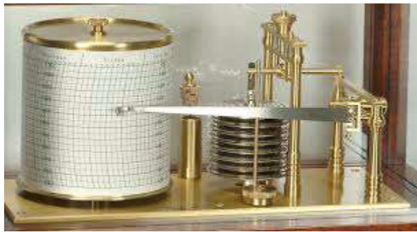
FIGURE 1. Typical Mechanical Barograph
