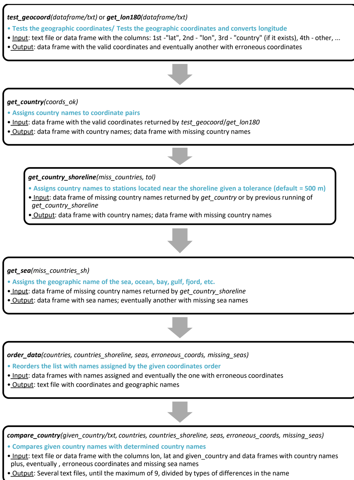
Fig. 4. Workflow, concept and relation among functions of the stlocationqc software.
